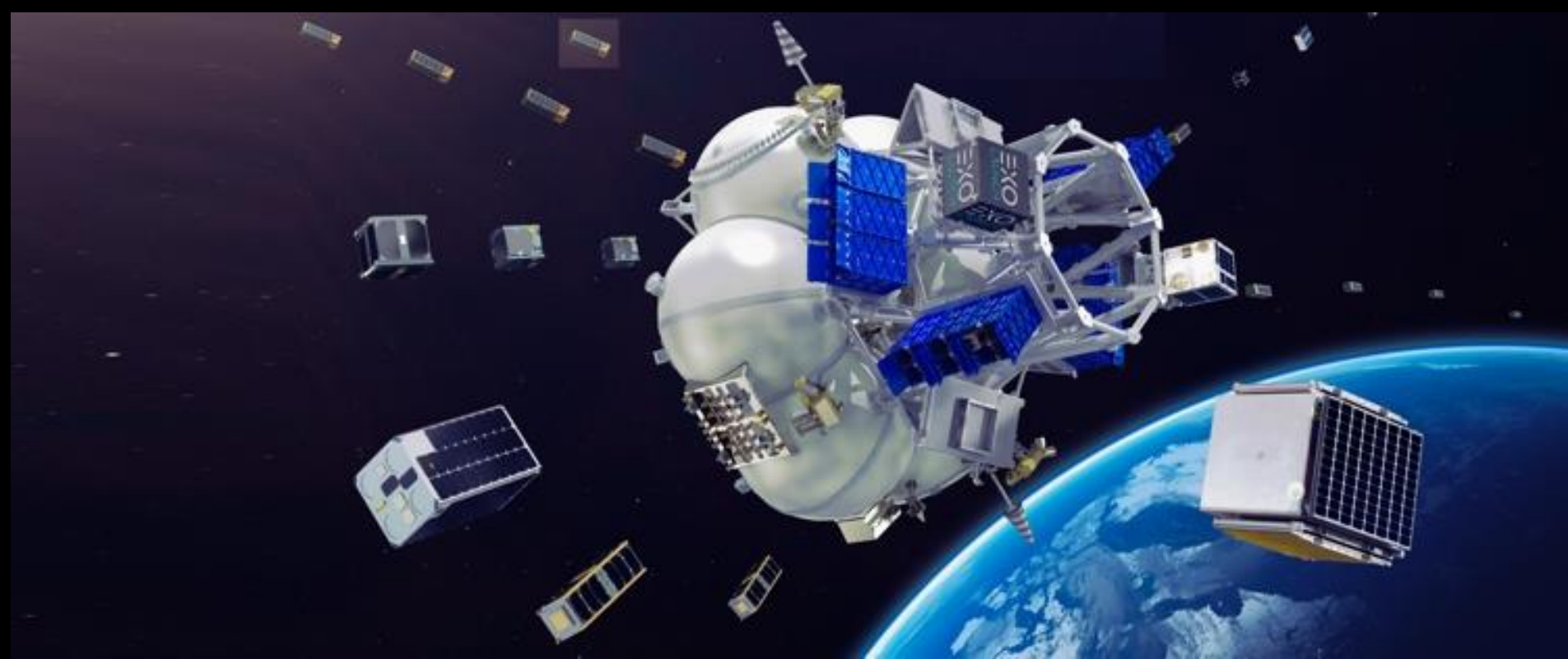
Artist's illustration of small satellites deploying from Soyuz rocket's upper stage. Credit: Exolaunch
